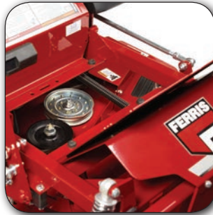
Turn the removable floor pan knob to gain access to the top of the deck when maintenance is needed.
