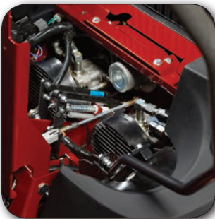
Fans mounted on side of pumps assist in cooling of hydro system and repelling debris.
