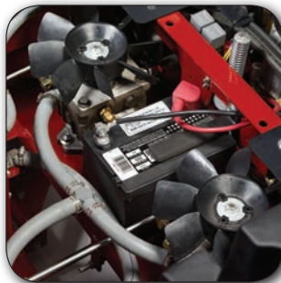
8" fans mounted on top of pumps assist in cooling of hydro system and repelling debris.
