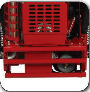
Heavy-duty integrated rear bumper protects engine compartment.
