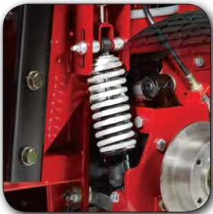
Suspension system consists of rear coil-over-shocks with dual cast-iron maintenance-free suspension arms (shown) and front independent adjustable shocks.
