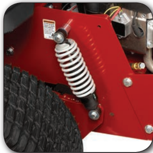
Suspension system consists of rear coil-over-shocks (shown) and pivoting front axle with coil-over-shocks.
