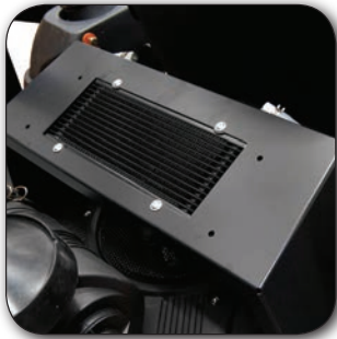
Transmission oil cooler for enhanced transmission longevity.
