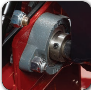
Pillow block bearings on control mounts makes for long lasting smooth, precision controls.
